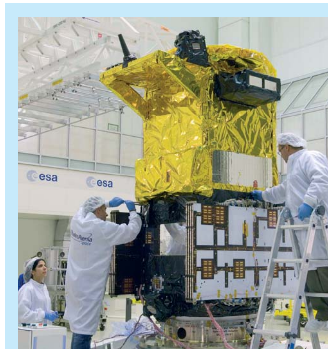
GLOVE-B, the second Galileo demonstration satellite, is prepared for vibration testing in the ESTEC Test Centre. Launch is planned for March 2008 on a Soyuz rocket from Baikonur Cosmodrome in Kazakhstan
